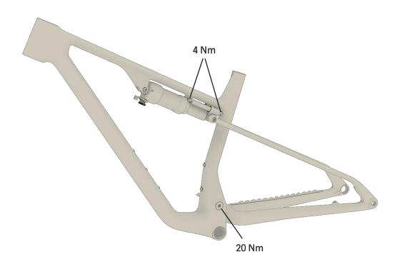
Unless otherwise noted, all bolts on the Silva frame should be tightened to 5 Nm, and Loctite 222 should be applied before reinstalling the bolts.
