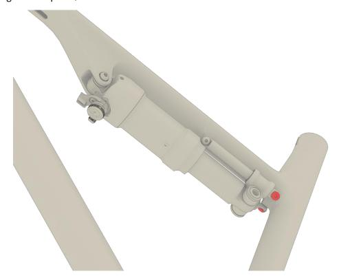
Now, remove the front shock mount bolt and tilt the shock down. Loosen the two bolts at the front of the rails (marked in red below) and move the slider forwards. Tighten the front bolts to 4 Nm.
